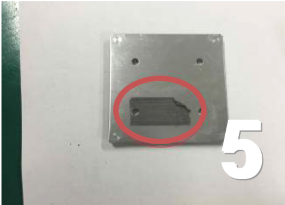
Remove residual tape on the back-plate.
