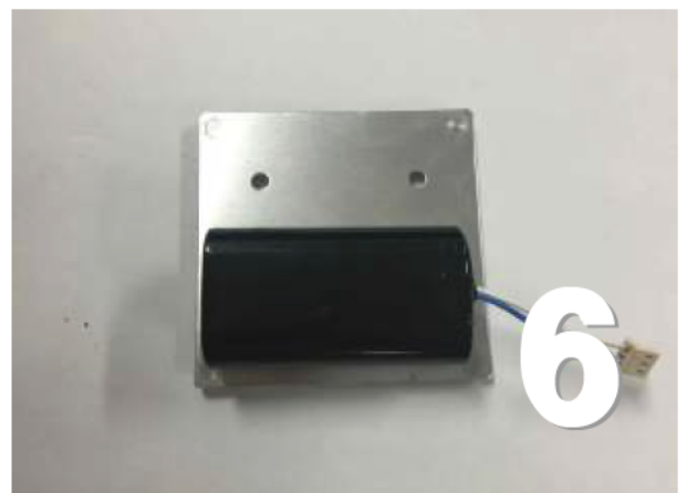
Remove backing on the two way tape from the new battery; center carefully on the two holes and make a little space between two batteries.
